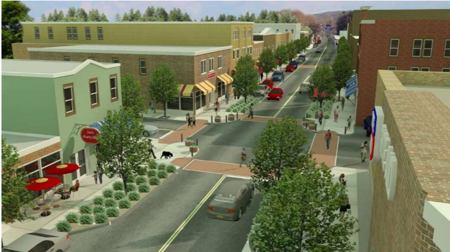
The integration of rain gardens and bioswales in extended bumpouts help contain and drain flood water.
