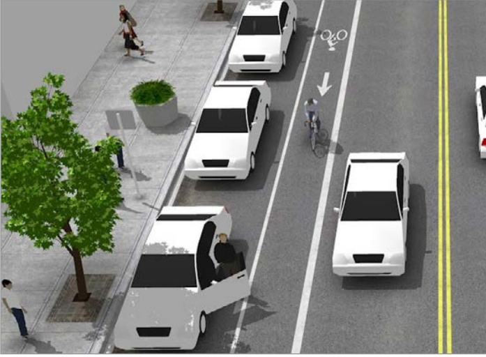
On-street parking can be employed as a buffer to the sidewalk. Adjacent bike lanes should be wide enough to avoid “dooring” accidents.
