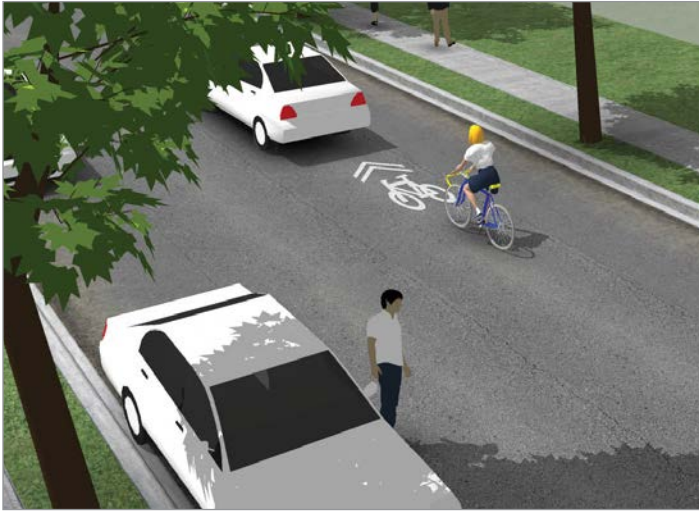
Shared lane markings help to position the bicyclists in the travel lane. (Source: NACTO)
