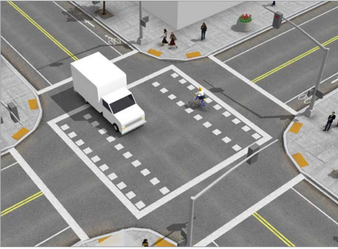
Intersection crossing markings identify where bicyclists should cross. (Source: NACTO)
