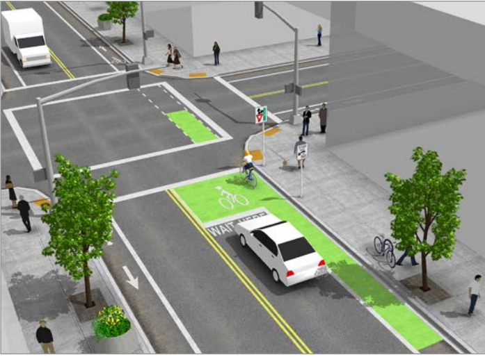
Bike boxes place bicyclists ahead of motor vehicle traffic at intersections. (Source: NACTO)
