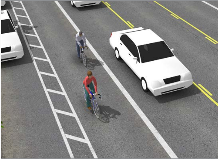
Bike lanes can be striped adjacent to parking or adjacent to the curb. When adjacent to parking, a striped buffer area minimize the occurrence of “dooring” accidents. (Source: NACTO)
