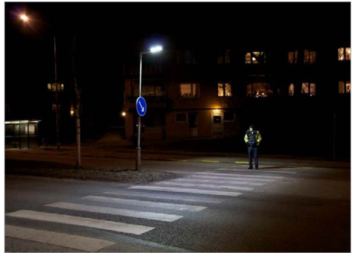
At this mid-block crossing, the pedestrian is illuminated for oncoming vehicles. (Source: LowerEnergyDesigns.com)
