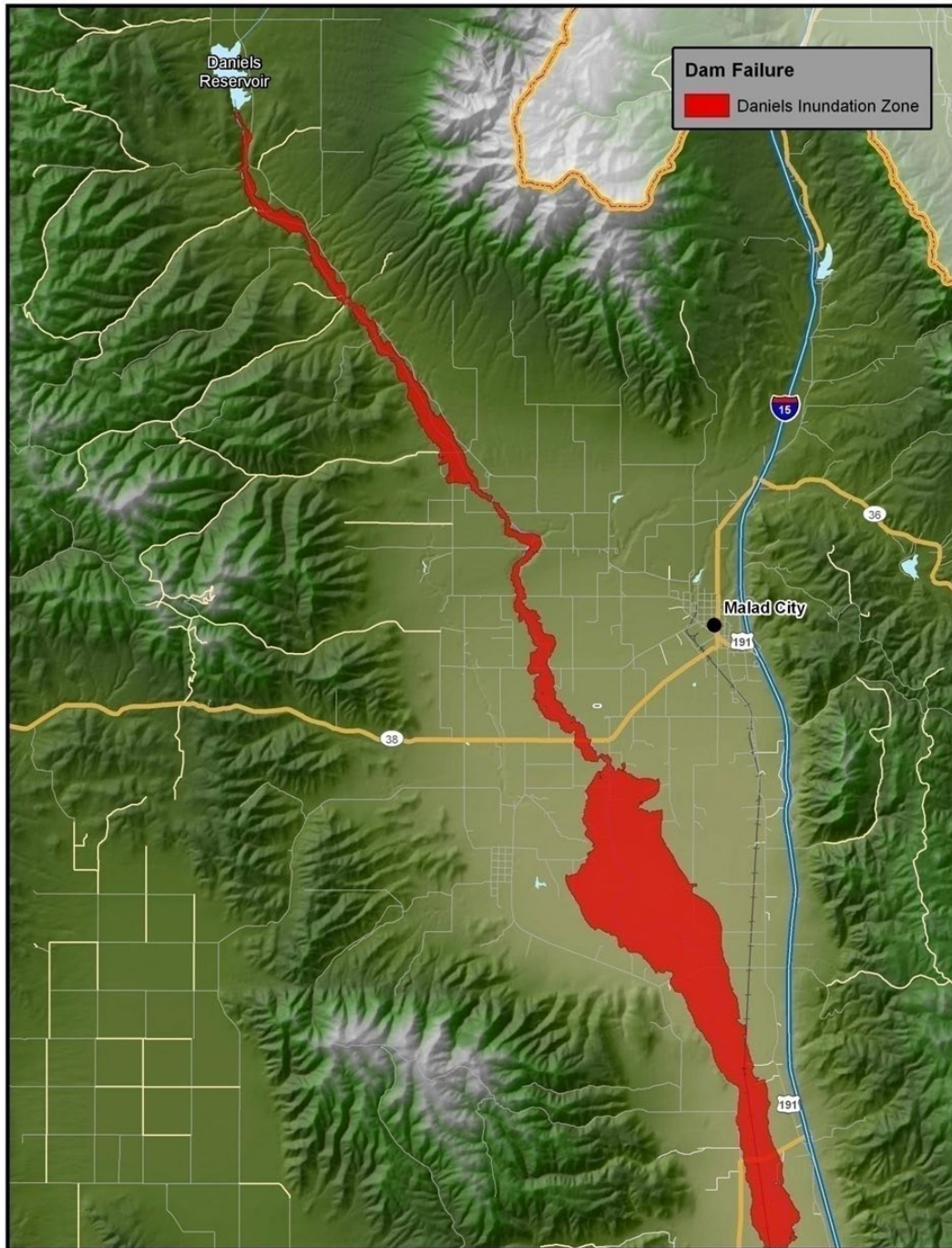
Figure 7-4. Daniels Dam Failure Map
