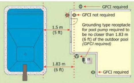
At least one general-purpose receptacle is required between 1.83 m (6 ft) and 6.0 m (20 ft) at permanently installed outdoor pools/spas
