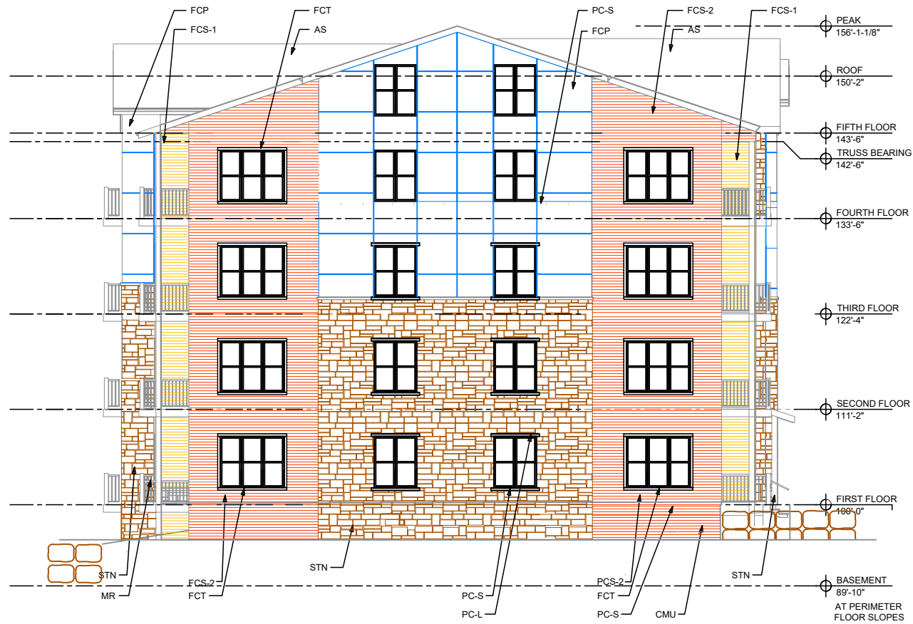
② WEST ELEVATION 1/8" = 1'-0" ON 22x34 HALF SCALE ON 11x17
