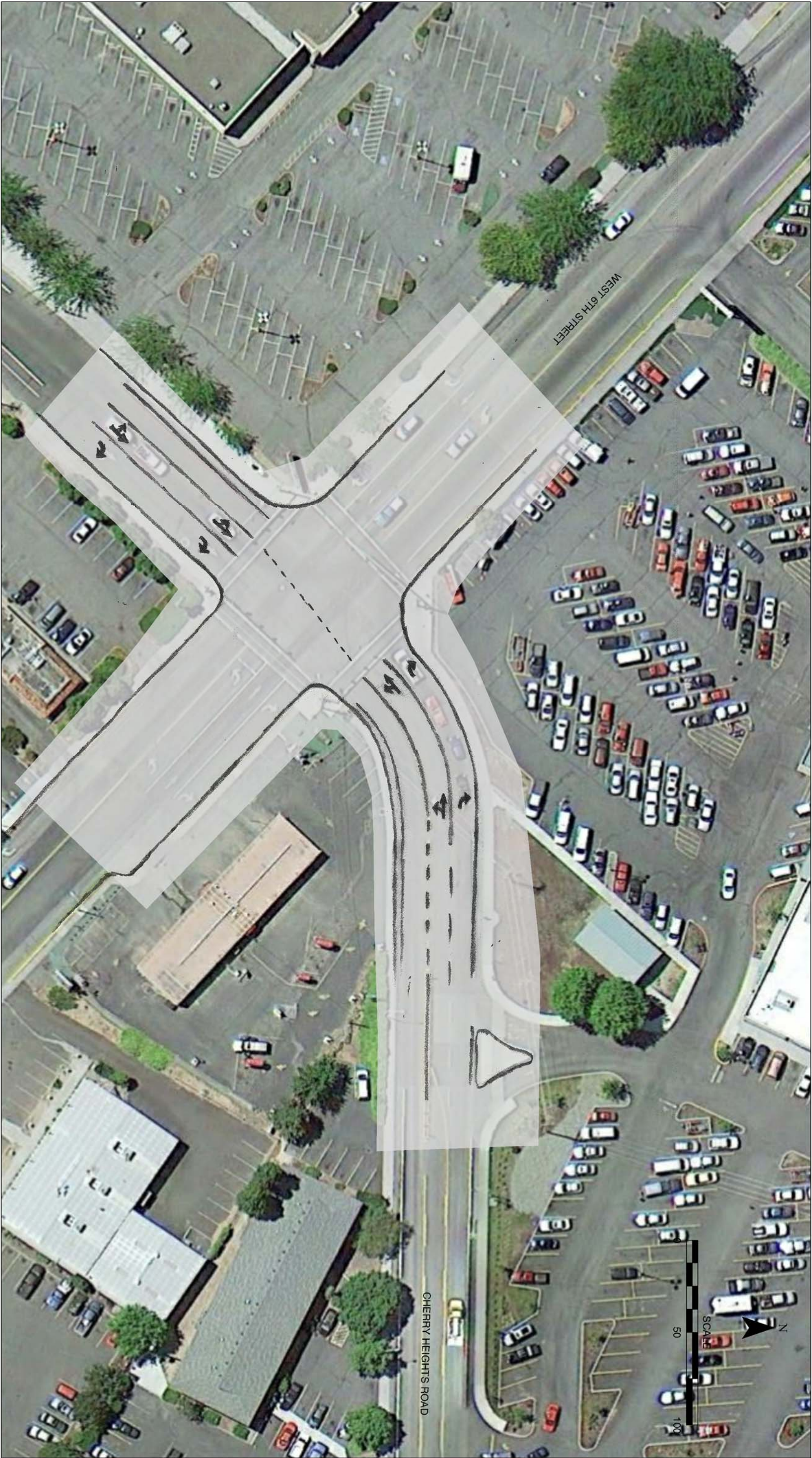
PROJECT I-8: CONCEPTUAL LANE RESTRIPIING CHERRY HEIGHTS ROAD/W 6TH STREET THE DALLES, OR Figure 5-9
