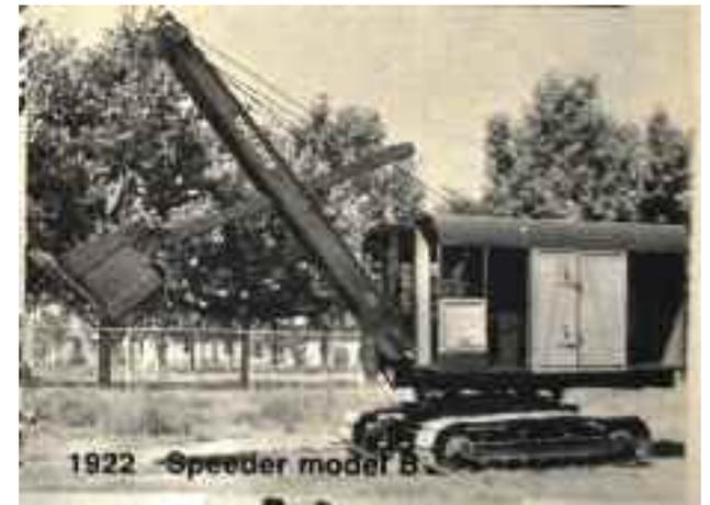
**Figure 4.** Early Speeder Model B Shovel Crane produced at the Fairfield, Iowa Speeder plant in 1922. From Link-Belt Cranes Booklet circa 1985, p. 19. (Courtesy of Carl & Mary Koehler History Center).
