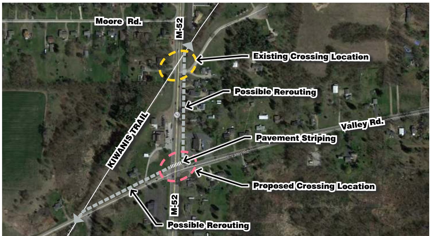
Above: M-52/Adrian Highway - Kiwanis Trail Crossing
