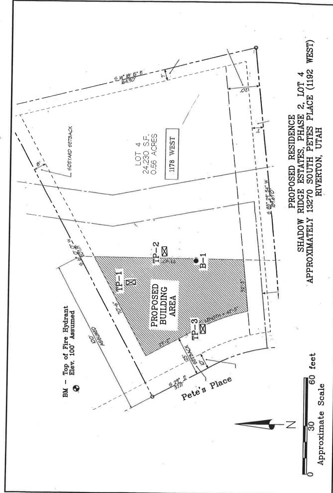
Locations of Exploratory Boring and Test Pits
