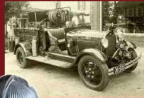
1929 Ford engine with a front mount pump—the company's first motorized apparatus. Now owned by the Rocky Ridge Volunteer Fire Company.
